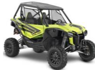
2-Person Talon R 104HP / 70MPH 6-Speed Shaft Drive DCT Automatic
